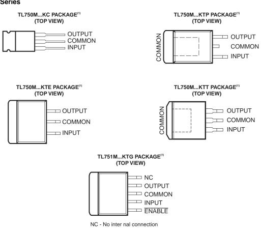
(1) The common terminal is in electrical contact with the mounting base.
