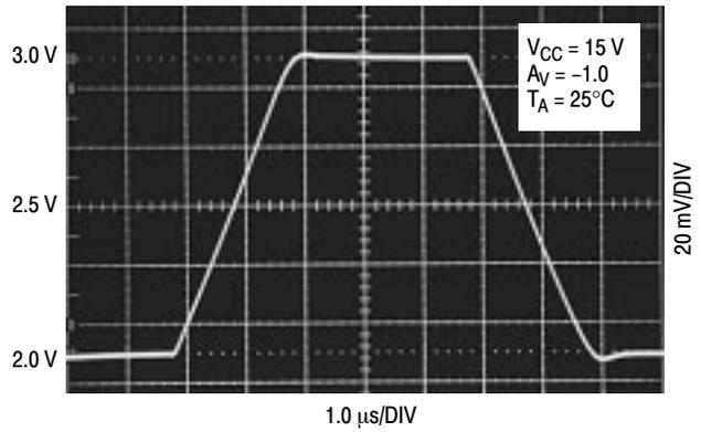
Figure 7. Error Amp Large Signal Transient Response
