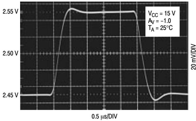
Figure 6. Error Amp Small Signal Transient Response
