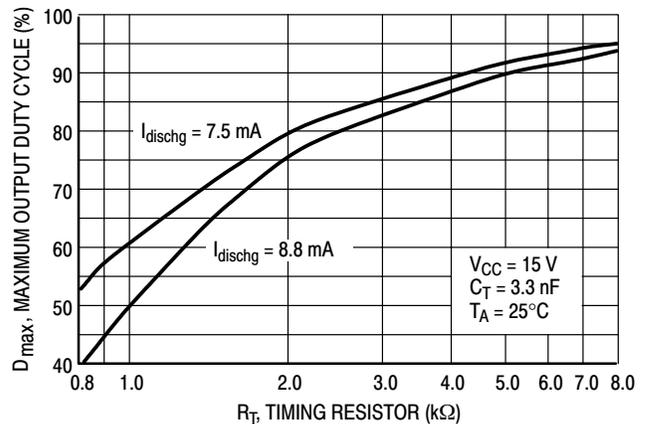
**Figure 5. Maximum Output Duty Cycle versus Timing Resistor**
