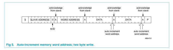
Page write: The PCF8582C-2 is capable of an eight-byte page write operation. It is initiated in the same manner as the byte write operation. The master can transit eight data bytes within one transmission. After receipt of each byte, the PCF8582C-2 will respond with an acknowledge. The typical E/W time in this mode is  $9 \times 3.5 \text{ ms} = 31.5 \text{ ms}$ . Erasing a block of 8 bytes in page mode takes typical 3.5 ms and sequential writing of these 8 bytes another typical 28 ms.
