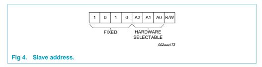
The last bit of the slave address defines the operation to be performed. When set to logic 1, a read operation is selected, while a logic 0 selects a write operation.
