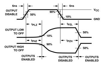
FIGURE 4. HC THREE-STATE PROPAGATION DELAY WAVEFORM
