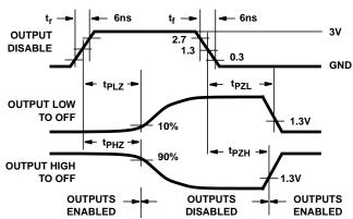
FIGURE 5. HCT THREE-STATE PROPAGATION DELAY WAVEFORM
