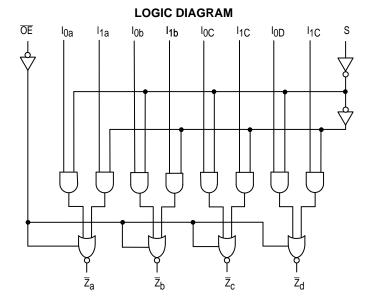
**MC74F258A QUAD 2-INPUT MULTIPLEXER** WITH 3-STATE OUTPUTS FAST™ SCHOTTKY TTL **J SUFFIX** CERAMIC CASE 620-09 **N SUFFIX** PLASTIC CASE 648-08 D SUFFIX SOIC CASE 751B-03 **ORDERING INFORMATION** MC54FXXXAJ Ceramic MC74FXXXAN Plastic MC74FXXXAD SOIC LOGIC SYMBOL 1
